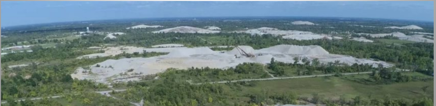
“chat” - silica waste left over after removal of Pb/Zn ore – Picher, Oklahoma
